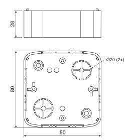
product description: designed for distribution system with voltage 400 V and with maximum current 16 A intended for devices of Tango - ABB series suitable for devices with great mounting depth on the sides of the box are marked inlets for the trunknings to install on materials with fire classes E or F, use insulating pad can achieve IP 40 while used with cover VLK 80/T
