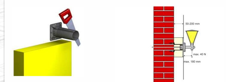
There is necessary to cut the carrier including inserted insulation before installation depending on layer thickness insulation.
