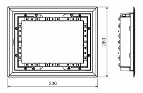
The complete assembly of the PP 80/K-5 and KUP 80 pulling floor boxes is designed for concrete floors where there is a need for branching or
